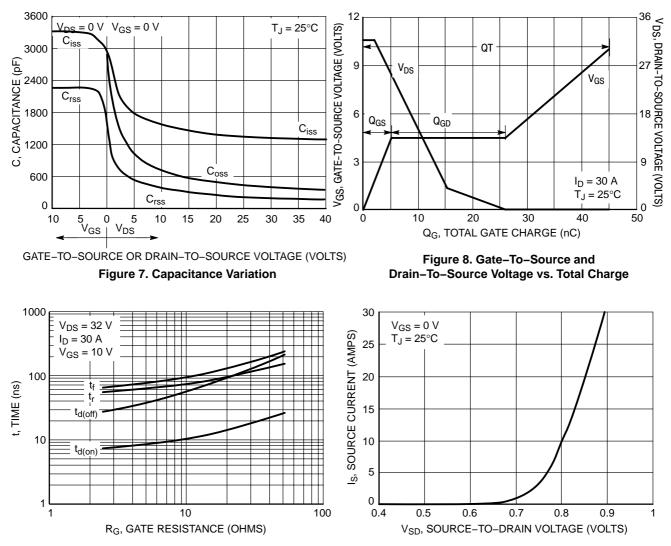
Figure 9. Resistive Switching Time Variation vs. Gate Resistance
